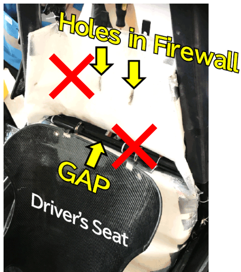
Firewall に穴や隙間のある例 Example of holes and gap in the firewall
