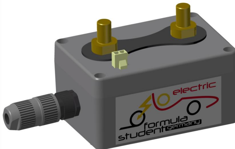
Figure 1: FSE2014 Energy Meter CAD Rendering
