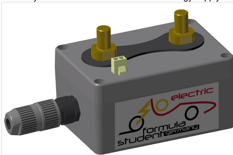
Figure 1: FSE2014 Energy Meter CAD Rendering
