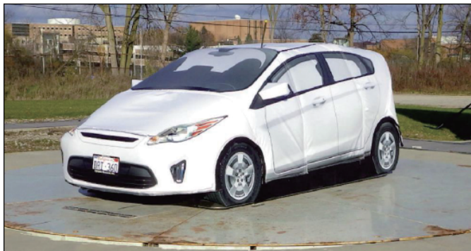
Figure C.6 — Example measurement cart (top), turntable (bottom)
