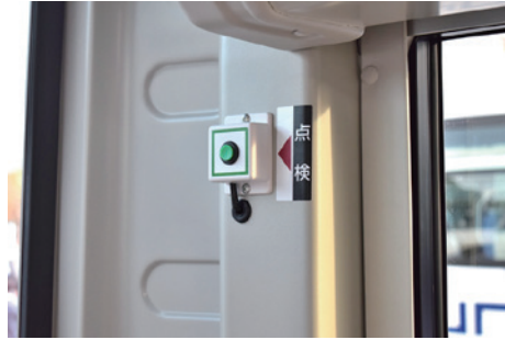
Fig. 16 Example of Device to Prevent Leaving Someone Behind on the Bus (Switch)
