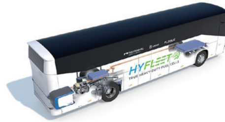
Fig. 8 Image of Integrated Powertrain and FC Module Jointly Developed by ZF and Freudenberg
