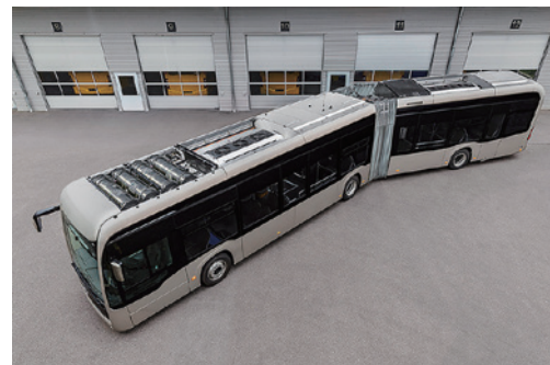
Fig. 4 Mercedes-Benz eCitaro Range Extender Equipped with Toyota's Second-Generation FC Module
