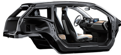
Fig. 2 BMW i3 passenger cell made from CFRP (source: BMW website).
