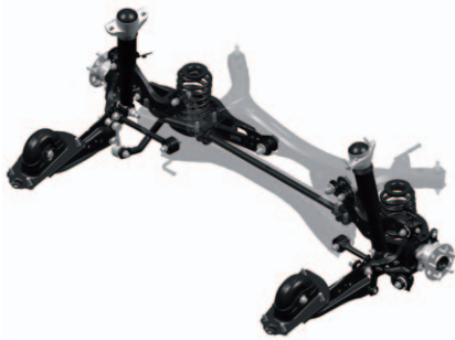
Fig. 1 Toyota Double Wishbone Rear Suspension (The figure shows the suspension of the Prius (4) )
