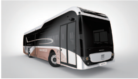
Fig. 29 Ebusco 3.0 Featuring a Composite Body and Cruising Range of 500 km on One Charge
