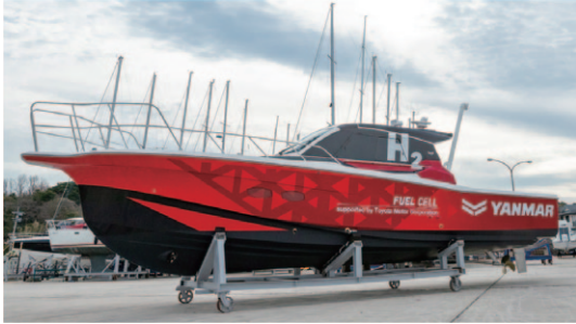
Fig. 6 Yanmar Maritime FC System Demonstration Test Boat
