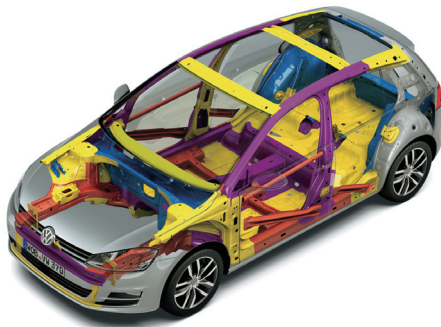
Fig. 7 Image of stiff sections of the Volkswagen Golf body.
