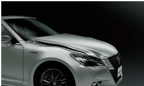
Fig. 4 Pop-up hood of the Toyota Crown.
