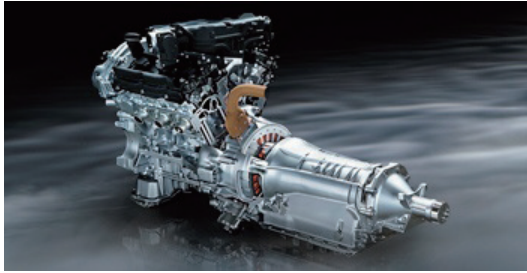
Fig. 7 1-motor, dual-clutch hybrid system of the Cima.
