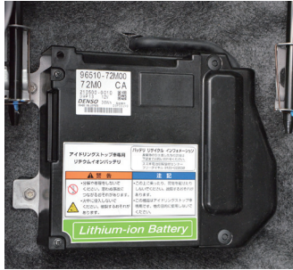
Fig. 21 The ENE-CHARGE lithium-ion battery is located below the front passenger's seat.
