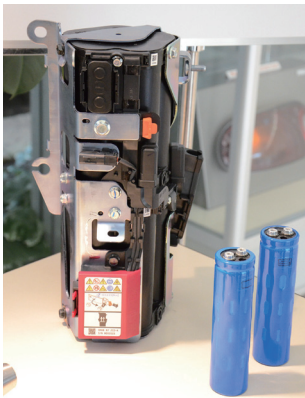
Fig. 13 Capacitors that store regenerated energy.
