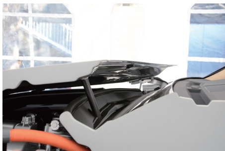
Fig. 3 Pop-up hood that contributes pedestrian protection.
