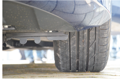
Fig. 23 Underbody aerodynamic parts on the Mercedes-Benz B Class.
